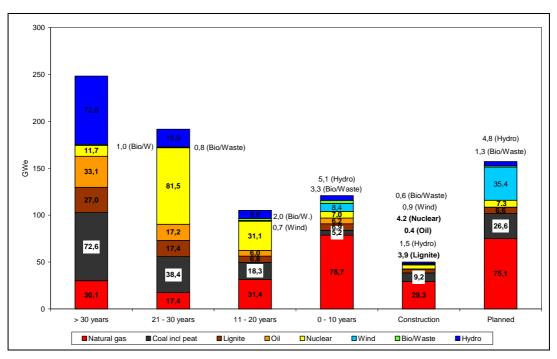
figure 1: operating and planned power plants capacity in EU-27 by fuel and age [6]
