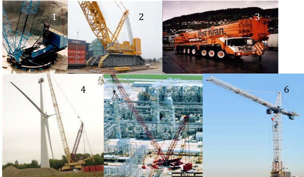
Figure 1: Types of mobile cranes
