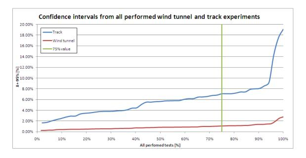
With the wind tunnel experiment it is in 75% of all experiments possible to distinguish a difference between two positions of 2.14% with a certainty of at least 95%. Compared to the 14.1% of the track experiment one can only conclude that, in this research, the wind tunnel experiment is far more accurate than the track experiment.
