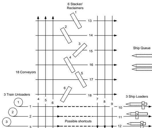
Figure 3: Schematic Terminal Lay Out with Equipment
