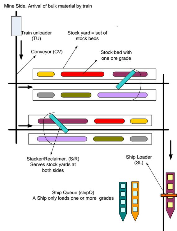
Figure 1: Terminal with Stock Yard and Stock Bed Lay Out
