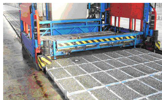
Figure 2b. A real (un)loading mobile robot, driving over a lane with racks containing trays with plants. (Florensis 2005)
