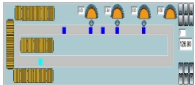
Figure 2. Animation screen of the pre-buffer model with 4 working stations and 3 mechanics. The pre-buffer assembly is split up in four steps. Each product is completed by one mechanic who steps along the working stations. The parts are supplied in one cart for each product. On the left side the loading of the assembly carts is represented.
