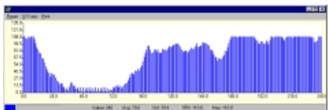
Figure 8: Contents of the decoupling buffer with a fixed number of 4 mechanics during 240 working days derived from a reverse time simulation run
