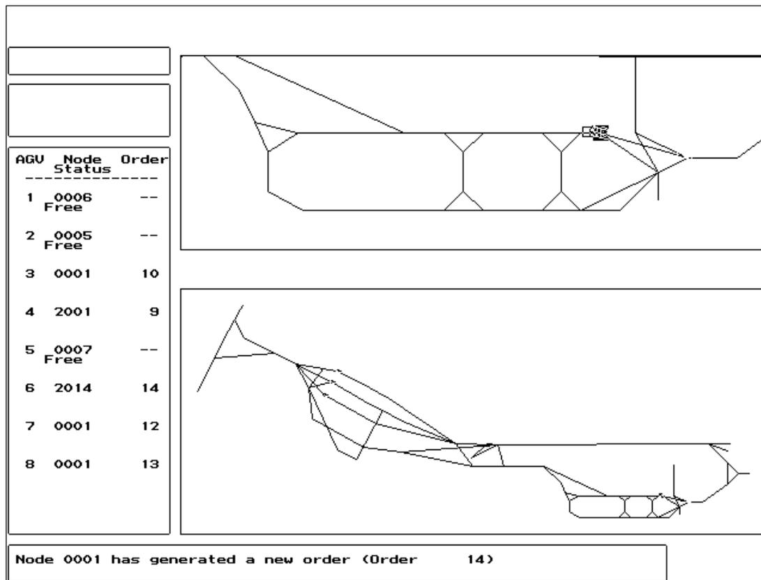
Figure 1: Capture of the simulation screen of an AGV system. The layout and routing are designed using a CAD tool called the Route Editor, the results of which are directly used for the simulation layout and for the AGV guiding. The upper part of the picture shows a magnified section of the lower part.
