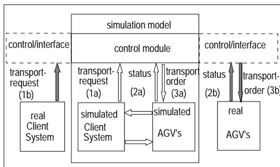
Figure 2: The simulation model working real time, controlling the AGV system. Real transport requests (1b) are now substituted for simulated transport requests (1a), transport orders are now going to both real AGVs (3b) and simulated AGVs (3a) and the simulated status is updated by the real status
