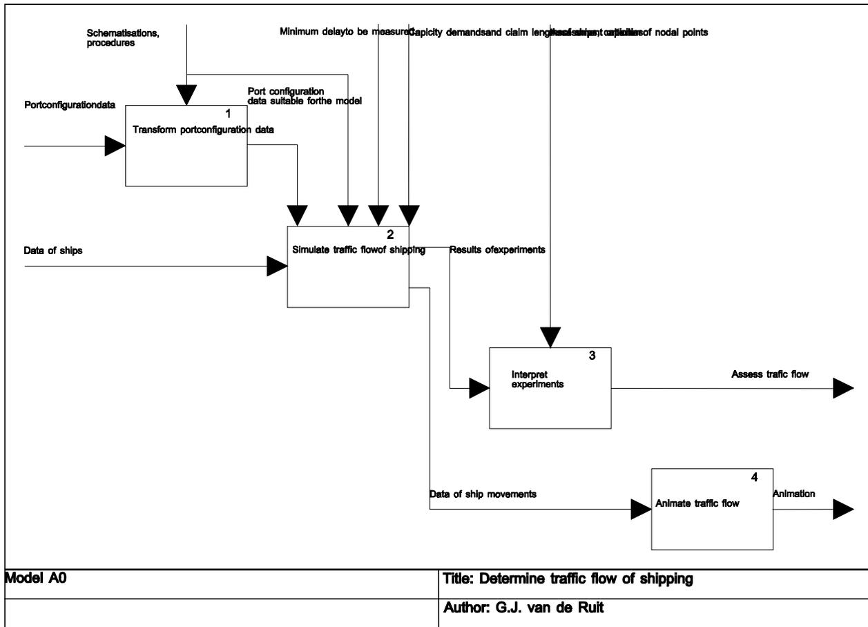
Figure 3 : Model A0 of the research project 'Traffic flow in the Maasvlakte'
